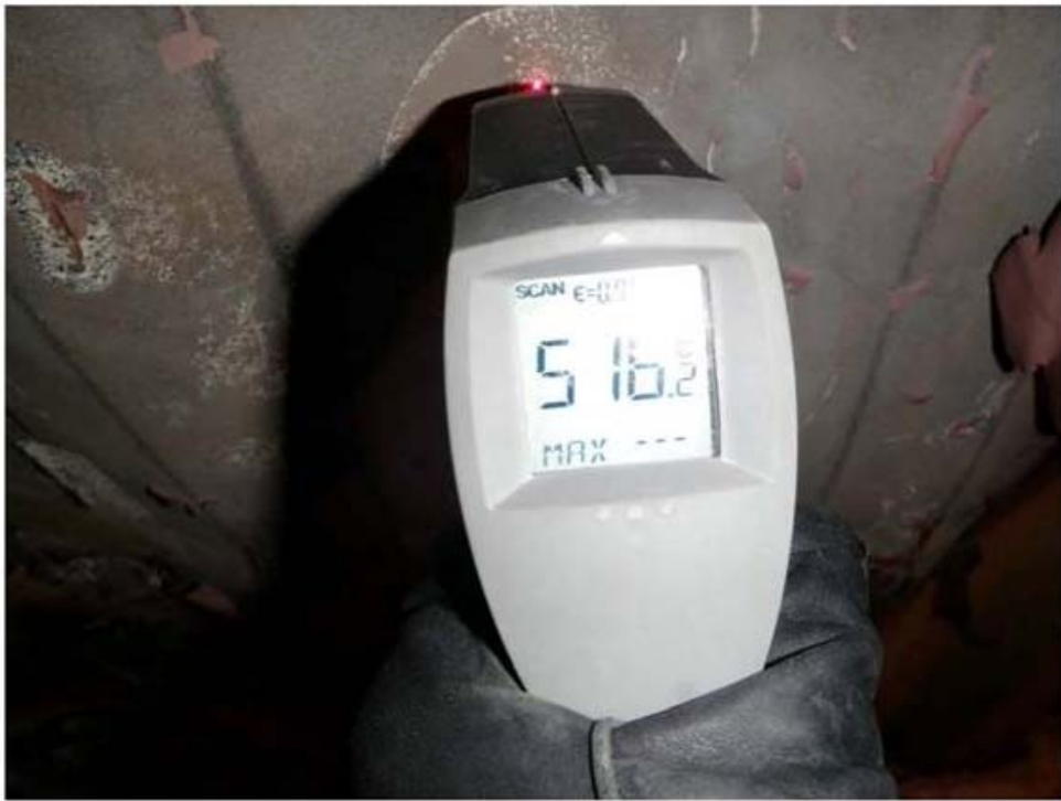
Temperature of 516°C on a hot spot on the outside of the container
